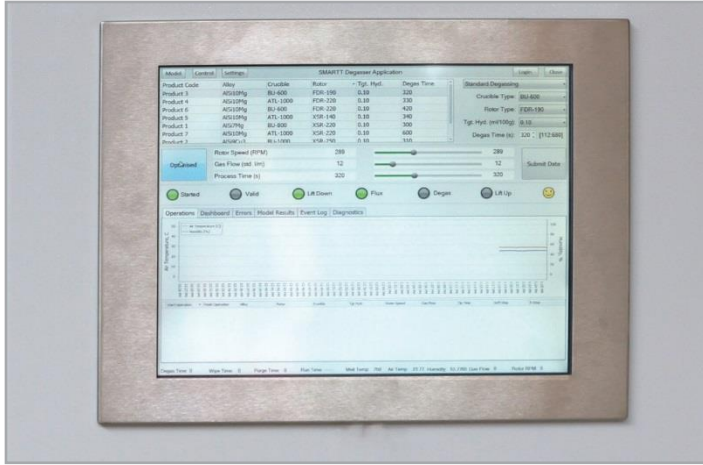
Picture 3: Touch screen interface in a FDU control cabinet door
