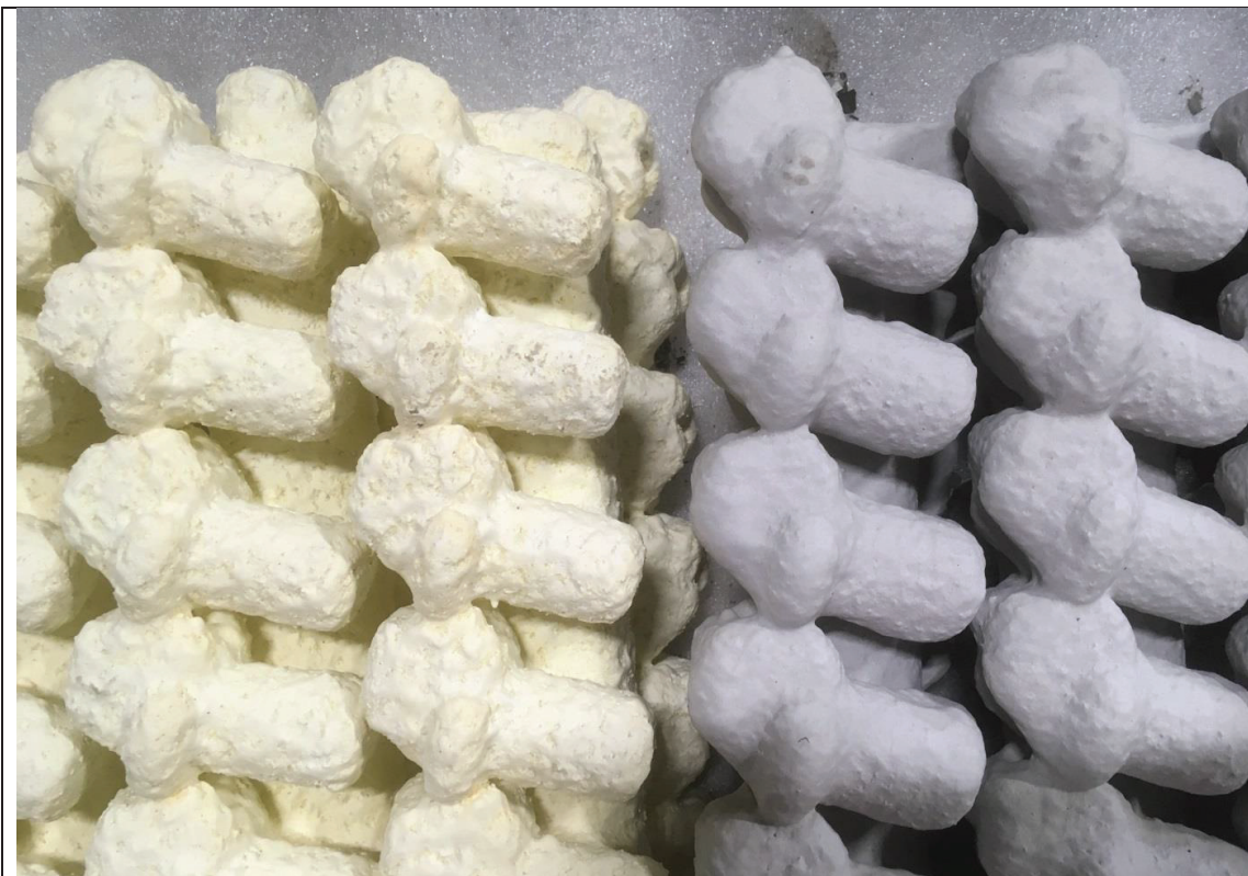
Fig. 3 Left: Aristo Cast standard shell, right: Hybrid+ shell. Both trees were built with one primary, three backups and a seal coat. Note the much thicker shell in case of using Hybrid+.
