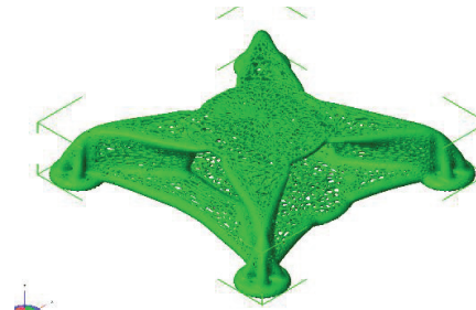
Figure 5 - Geometry 5, a lattice structure drone frame.
