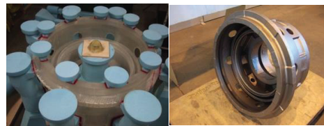
Figure 2 - Siemens Baring Chamber (SLA Hollow Pattern and Finished Casting)
