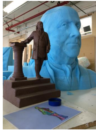
Fig. 15-17 CNC Milled White Polystyrene, 3D Printed Maquette and CNC Milling in Blue PIB
