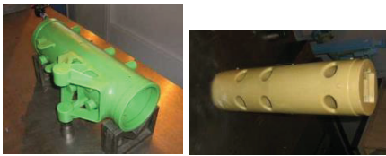
Figure 4 - Original Wax Pattern for Travel Lock Bracket with Enormous Soluble Wax Core
