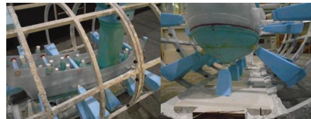
Figure 6 - Hybrid Pattern Process Combining Precision CNC PS with SLA for Galleon Designed by Ursae Ltd. to Commemorate the Birthday of William Shakespeare
