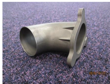
Figure 3 - Think Walled Exhaust Segment (Prototype SLA to Wax in Heat Resistant Ti-Alloy - Akrapovic)
