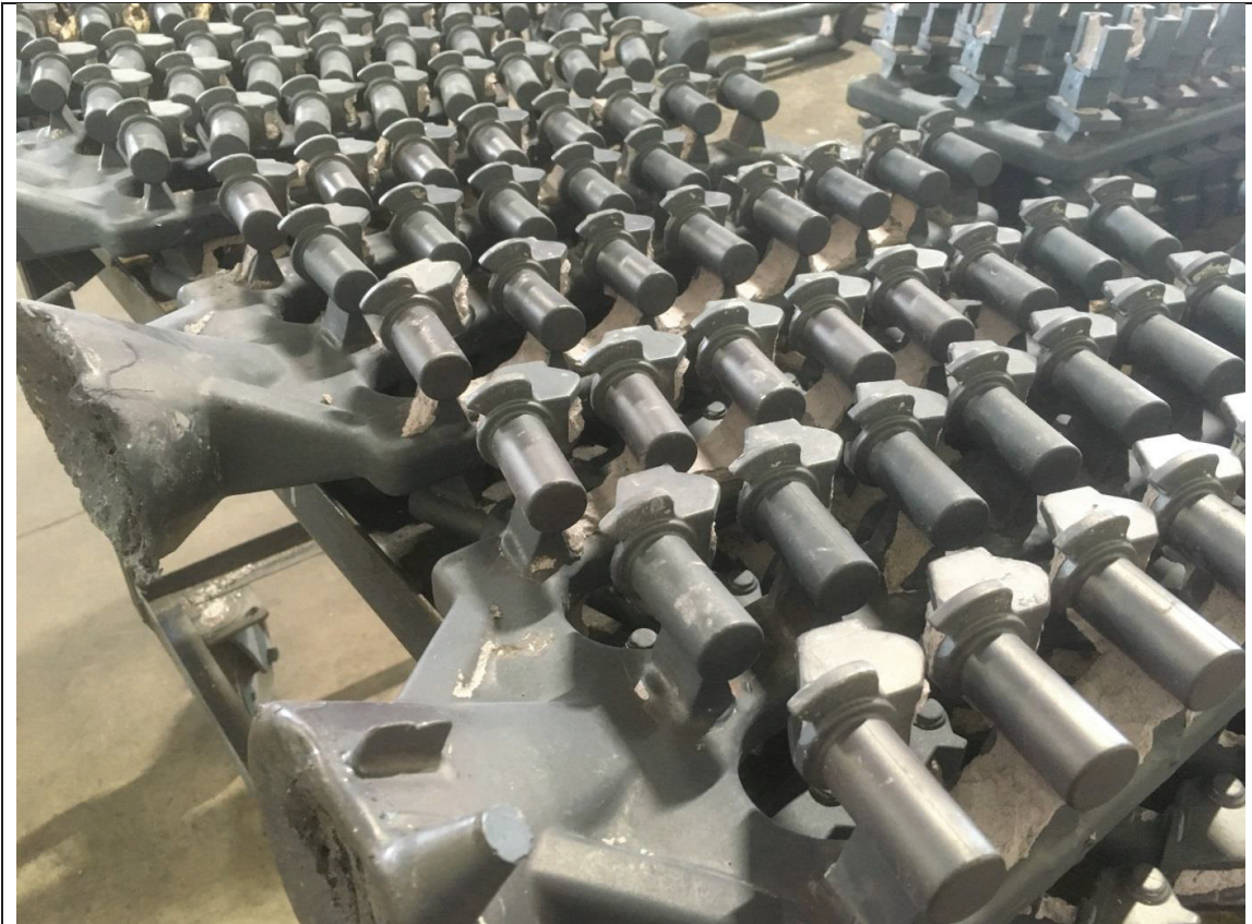
Fig. 5 Castings after shake out. Tree in the front: Hybrid+ shell, trees in the back: std. shell.
