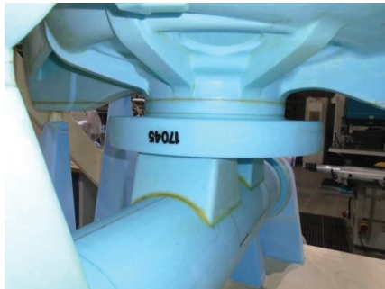
Figure 1- Precision Machined PS Replica (500kg Titanium Pump Casing)
